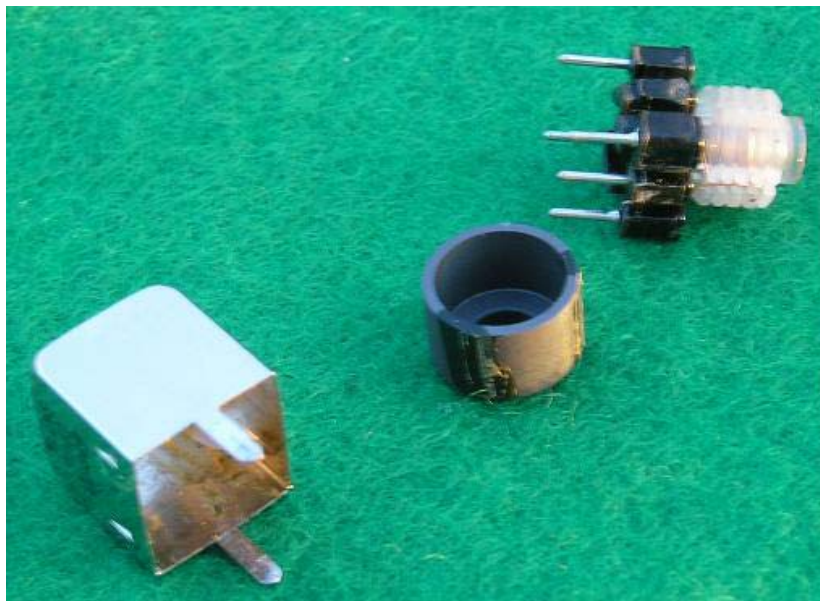
Fig 2 – the 10K Components – can, cup and bobbin
